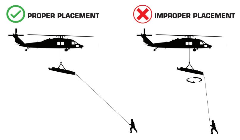
Proper placement prevent stretcher spin with minimum tension applied to tag line. Maximum visibility for pilot and ground crew. While better than no tag line at all, this placement of personnel and equipment tilts the stretcher, increasing the likelihood of spin and requires greater tension on the tag line to prevent the spin, creating an increased possibility of weak line separation.
