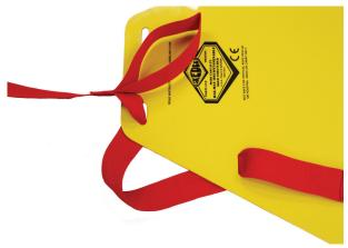
1. Lace the ends of the red tow strap with plastic handles through the slots at the head end. Start downward, then upward through the second slot.
