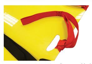
12. Attach the three extra slings provided with each HMH Sked<sup>®</sup>. They are used for easier handling when on stairways, steep terrain or to place the HMH Sked® onto a decontamination rack. They are attached by folding the sling at the line between the words FOLD | HERE on each sling. Insert the folded end through the cut-in hand holds of the HMH Sked<sup>®</sup>. Open a loop at the folded end. Insert the two sewn ends through the loop to form a girth hitch and pull it tight.
