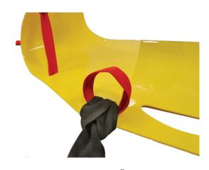
6. On each side of the HMH Sked® pass the loop end of the black strap through the red strap loop and through the adjacent slot in the HMH Sked®. Pull it through far enough to open the end loop and pass the buckle end of the strap through. This will form a girth hitch through the red strap end and the slot.
