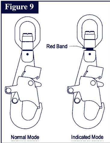
**Step 3.** See Figure 9. Inspect impact indicator on snap hook. If hook is in the indicated mode, return winch to an authorized service center for repair.
