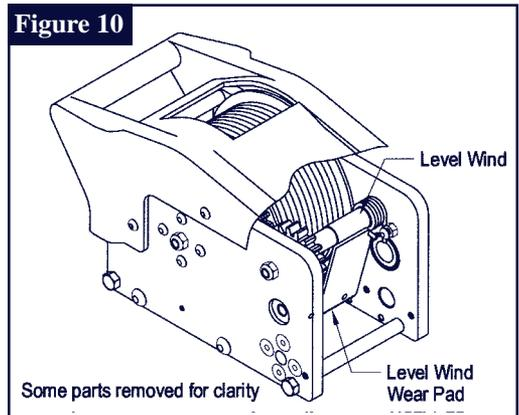
**Step 4.** See Figure 10. Inspect level wind assuring that it moves freely and applies pressure against the line. If the plastic wear pad needs to be replaced return the winch to an authorized service center.
