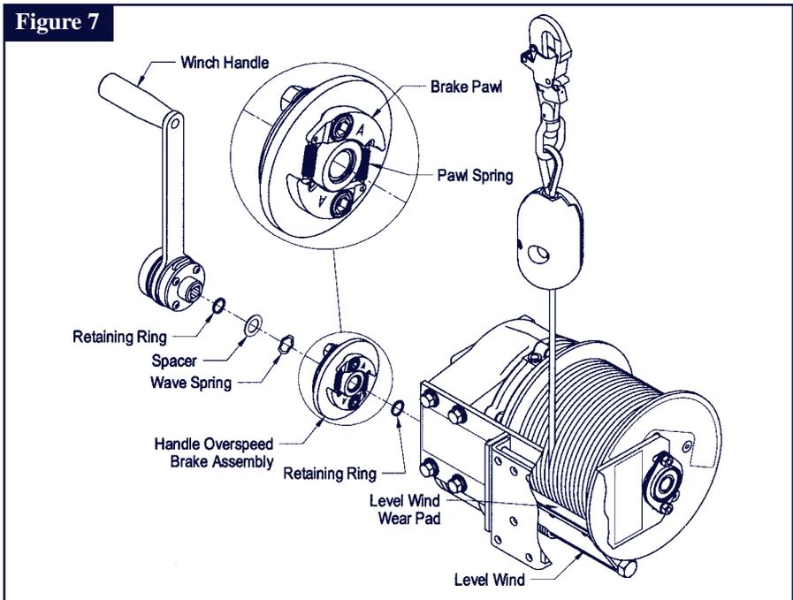
**Step 6.** See Figure 7. Inspect level wind assuring that it moves freely and applies pressure against the line. If the plastic wear pad needs to be replaced, return the winch to an authorized service center.
