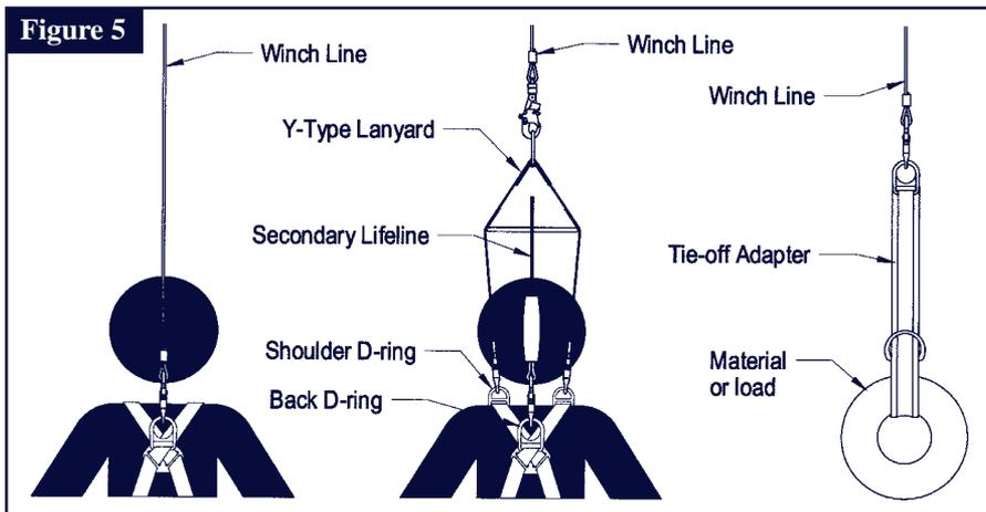
tached to the worker's harness shoulder D-rings. The secondary lifeline should be connected to the worker's harness back D-ring. For material handling applications, connect the winch line to the load using a tie-off adapter or other anchoring device.
